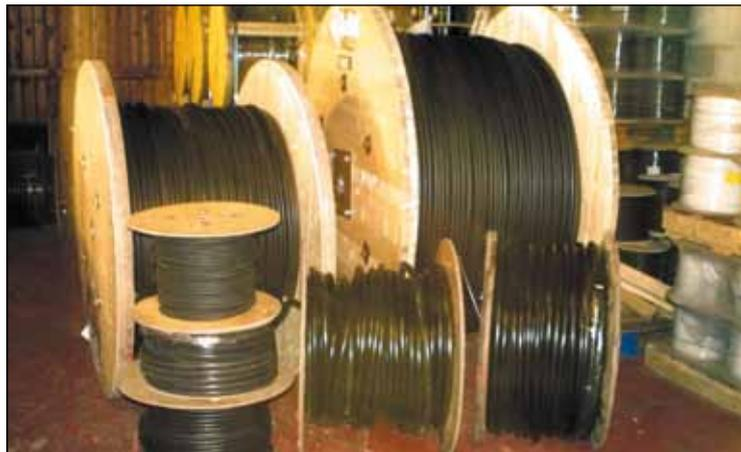
**CW 1128 external telephone cables - multipair, 0.5mm solid plain copper conductor, pvc insulated, jel filled, black polyethylene outer sheath. Suitable for installation in ducts or directly buried in suitably prepared ground.**
